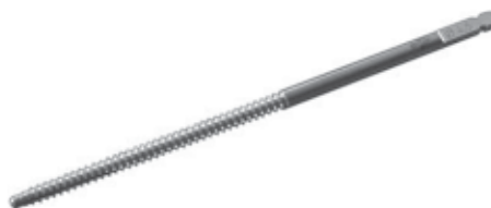
Tap for 4.5mm Cortex Screws ESC-66-007-01 Total length 125mm, thread length 70mm Predrilling: 3.2mm dia.
