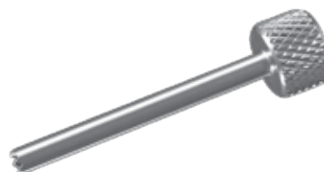
Insert Drill Sleeve 3.5/2.5 ESC-63-023-01 length 42mm, drill bit 2.5mm dia. For long 3.5mm lag screws
