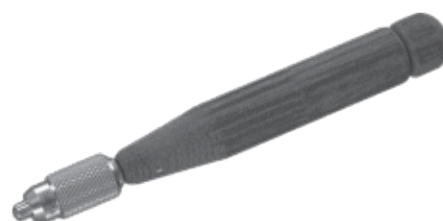
Hand Chuck for Kirschner Wires ESC-64-081-01 length 145mm, Spannbereich 0.6 to 1.6mm dia.
