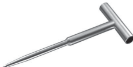
Screwdriver, hexagonal, with T-Handle, large ESC-62-023-01 to loosen tight screws. A normal screwdriver can be additionally inserted in the hollow shaft of the T-handle.
