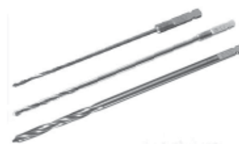
Drill Bits for quick coupling Drill bit 3.2mm dia.: for threaded hole of 4.5mm and 6.5mm Screws Drill bit 4.5mm dia.: for gliding hole of 4.5mm Screws
